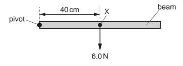
The beam weighs 6.0 N and its weight acts at a point X 40 cm from the pivot.
