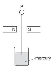
The wire is hanging vertically between the N and S poles of a magnet.
